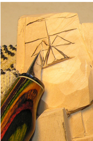
39. Cut towards the nose from the top of the eye corner down to the nostril to complete the chip cut.
