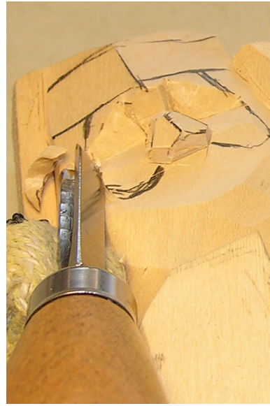
46. Using a V tool to chisel to cut with one blade away from the face.
